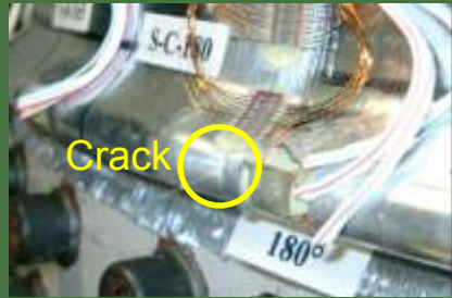
Crack (water leakage)
